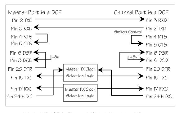
Master DCE / Sub-Channel DCE Interface Flow Diagram
